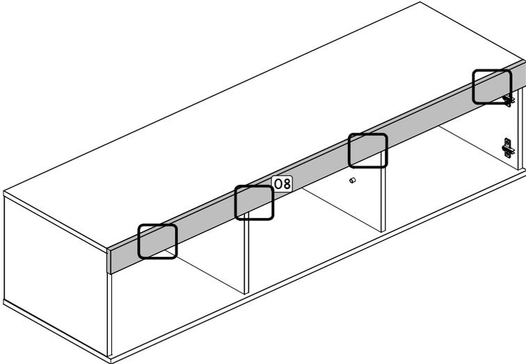
**Step 9:** Attach the backboard (11) using the hardware part I and a small mallet (not provided).
